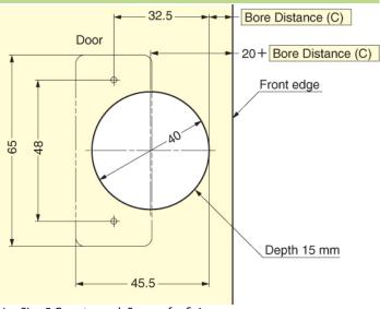
Use Size 5 Countersunk Screws for fixing.
