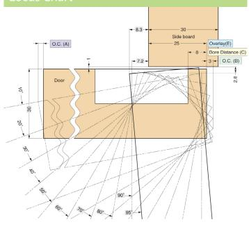
Clearance for door edge O.C. (A) and hinge side O.C. (B) are necessary. O.C. (A) and (B) change depending on door thickness and bore distance (C). Refer to locus chart and tables below when designing cabinets.
